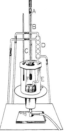
ture by the glass cylinder E, which rests upon the asbestos disk below and is covered with a detachable, stiff rubber cloth disk above.
